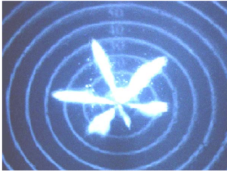
Figure 3-13. Photograph of the sprays with a six-hole VCO nozzle.
